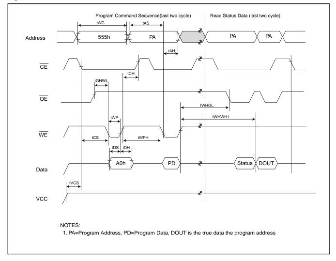
Fig 7. ACCELERATED PROGRAM TIMING DIAGRAM
